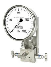
Differential pressure gauge with diaphragm element
