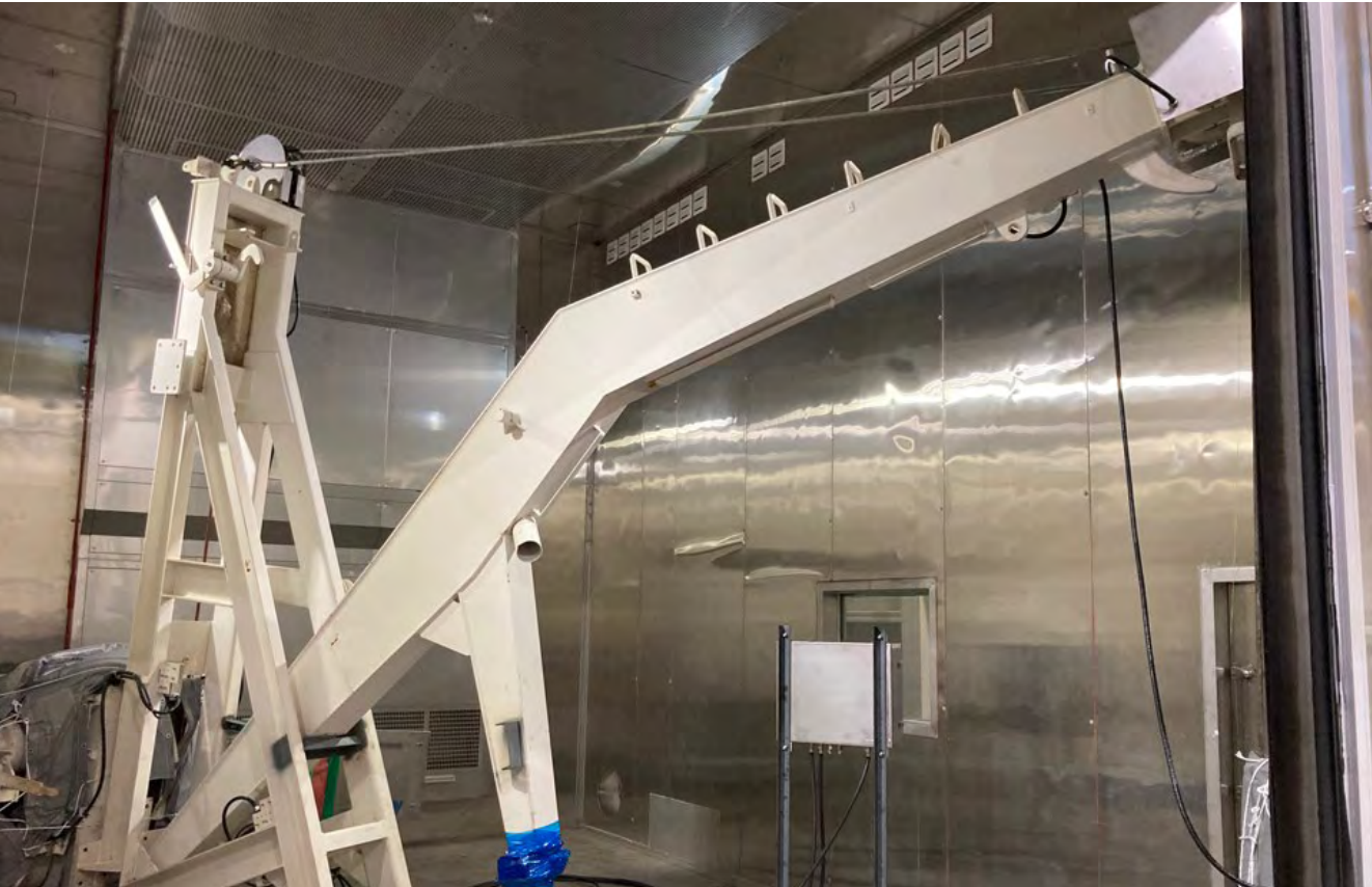
■ Lifeboat Davit Chamber Test under Extremely low temperature(-62°C)
