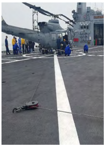
■ Helicopter Traversing System (3 winch 5 wire type & Rail type)
