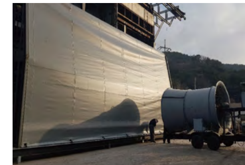
Wind test (Max. 30m/sec)
