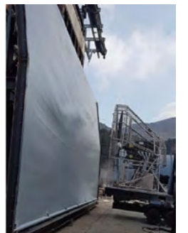
Wind test (Max. 30m/sec)
