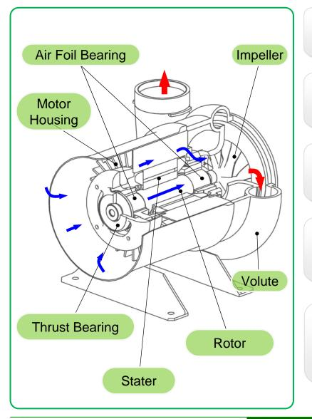
Extra cooling fan is not need for motor cooling(self cooling by)
